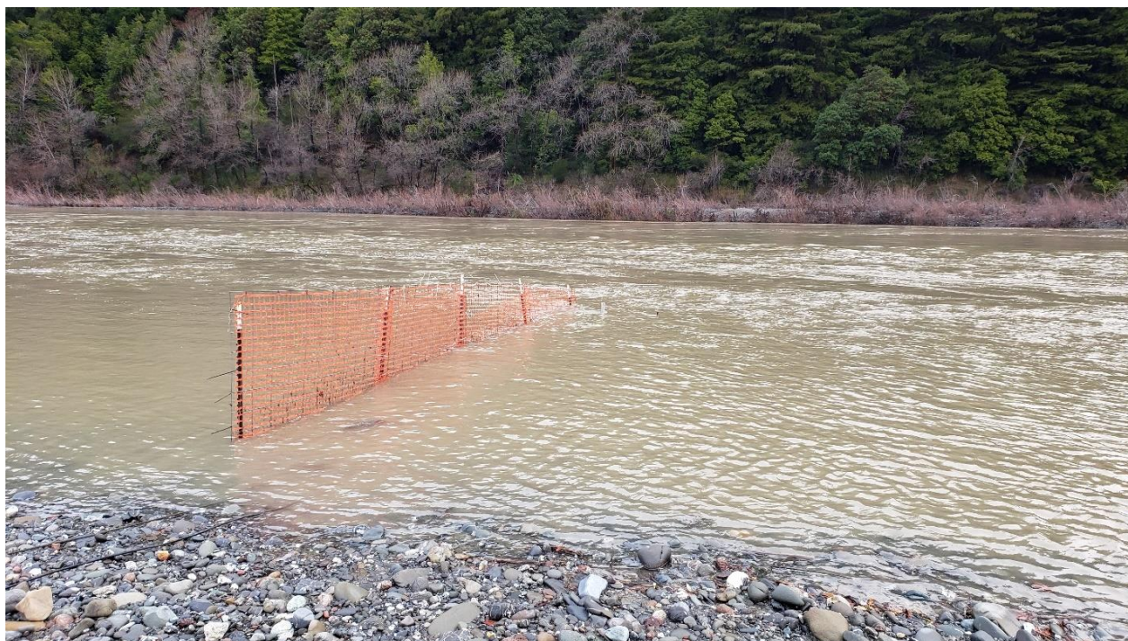
9.) 01.22.2020. Camera operating at near maximum depth and streamflow (7,630 cfs USGS Ft. Seward gage). Small temporary rock wall place behind closest panel.
