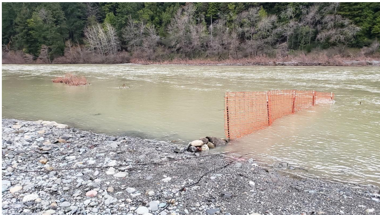
14.) 01.29.2020. Camera setup near maximum operational capacity. Rock wall constructed is approximately where 9,000 cfs brings water level to.
